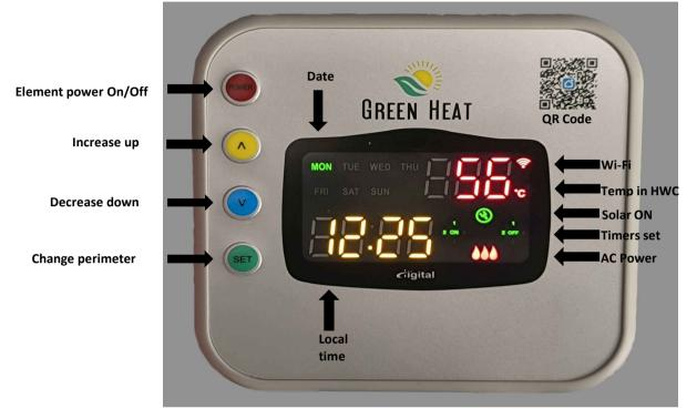
Element grid power can be turned ON/OFF with top red button (flashing = already on temperature and off)
