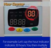
the number of hours with your HWC element rating, e.g. 4 kW. This then means that the user consumed 120 kWh since the last time the unit was reset.
