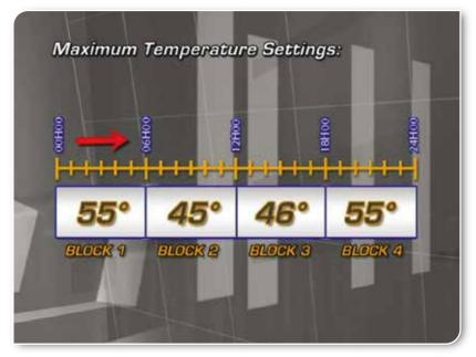
To adjust the maximum temperature settings, press the green button **repeatedly** until the first block temperature setting is displayed. The temperature will be flashing and the number of the block will be displayed in the timer indicator block. The below screens show the temperature flashing in block number 1.
