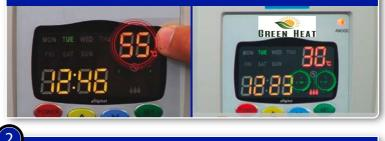
Set the temperature per block to user requirements by using  $\wedge$  and  $\mathbf{v}$  arrow keys.
